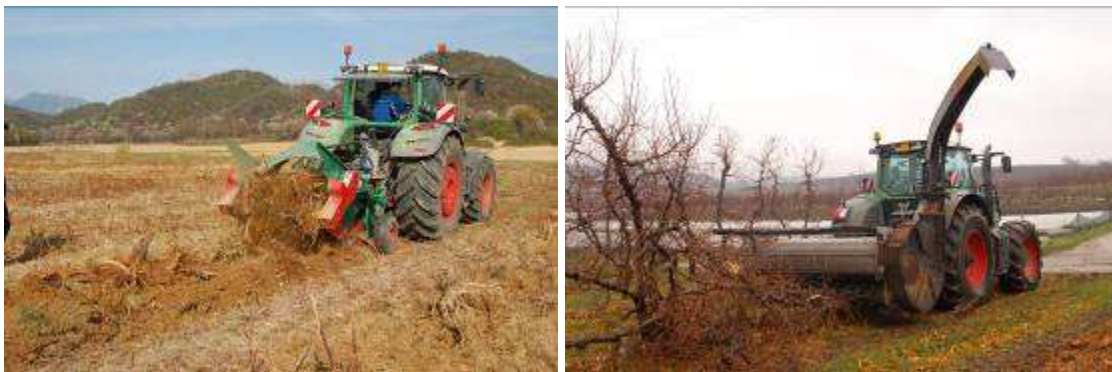
Figure 03-01 8: Examples of dedicated equipment for orchards uprooting by removal of the stumps (left) and one passage removal of the whole tree (right) (source: Gianni Picchi).
