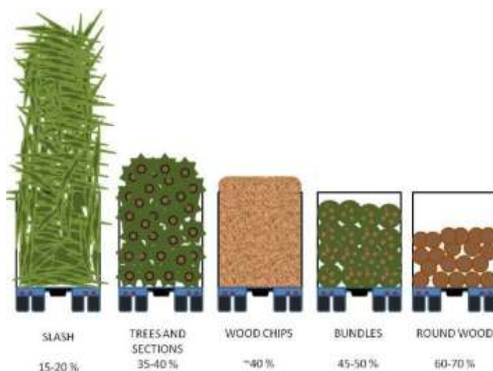
Figure 03-01 14: Bulk density of different assortments of forest biomass products compared to solid wood density (100%) and its influence on load efficiency.
