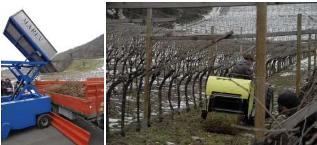
Figure 03-01 6: Dedicated harvesting equipment for agricultural pruning residues (source: Marco Fellin).
