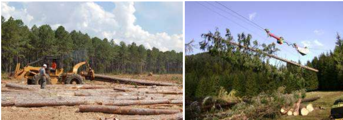
Figure 03-01 3: Skidder extracting manual felled and delimbed tree-length stems (left) and extraction of whole trees by mean of cable yarder on steep terrain (right) (source: Carolina Lombardini).
