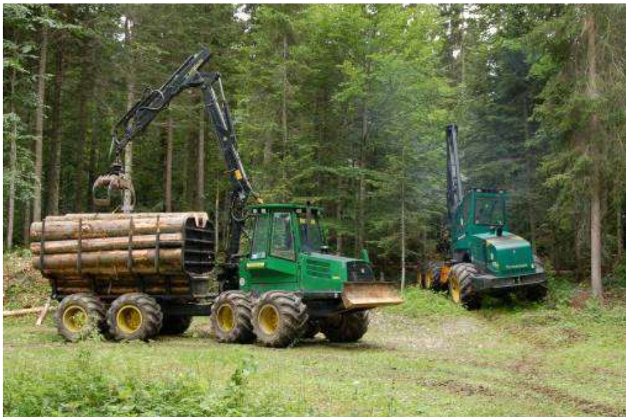
Figure 03-01 2: Forwarder (left side) loaded with processed logs, on the right side is visible the harvester used for felling and processing the trees (source: Gianni Picchi).
