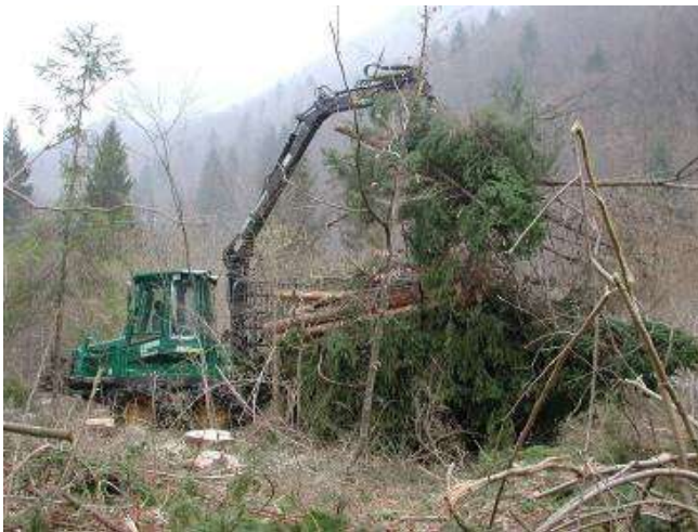
Figure 03-01 13: Extraction of loose residues by mean of forwarder (source Raffaele Spinelli).
