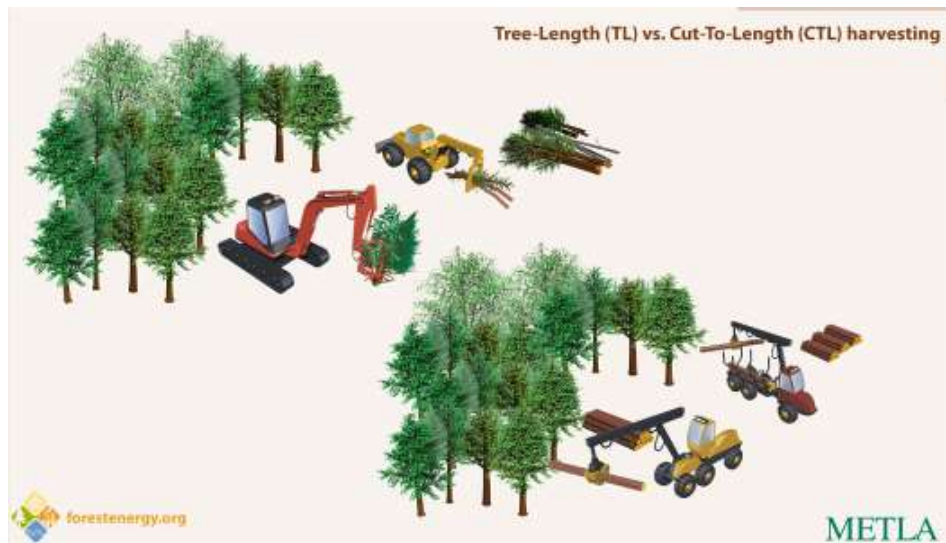
Figure 03-01 4: Schematic comparison of cut-to-length and tree-length systems (source: Forest Energy Portal).
