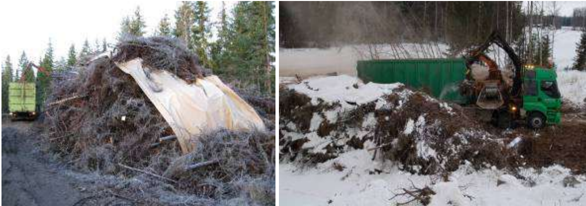
Figure 03-01 16: Forest residues piled at roadside and covered with biomass paper (left, Sweden), this cover type can be chipped directly with the woody biomass and delivered as fuel (right, Finland), facilitating the comminuting operation. (source: Gianni Picchi).
