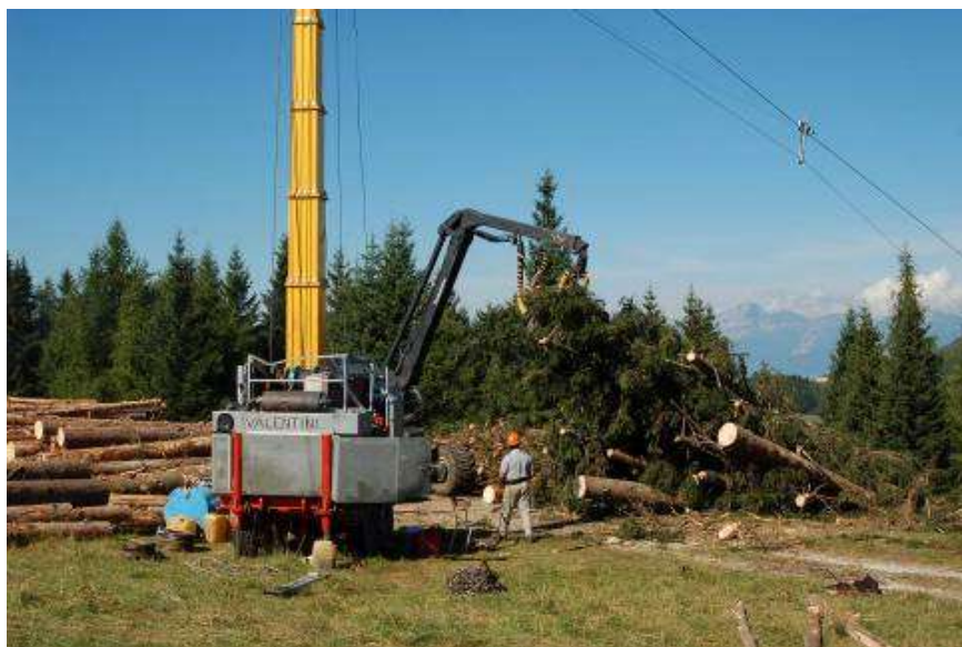
Figure 03-01 5: Extraction of tree section from the forest. Trees are processed on the spot, piling commercial timber and slash in different heaps. In order to clear up the landing it is important to promptly remove the piled material, this is the optimal point for residues transformation by chipping or bundling (source: Gianni Picchi).
