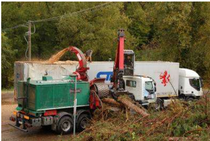
Figure 03-01 15: Chipping of whole trees loading the biomass directly on a high volume truck (source: Gianni Picchi).
