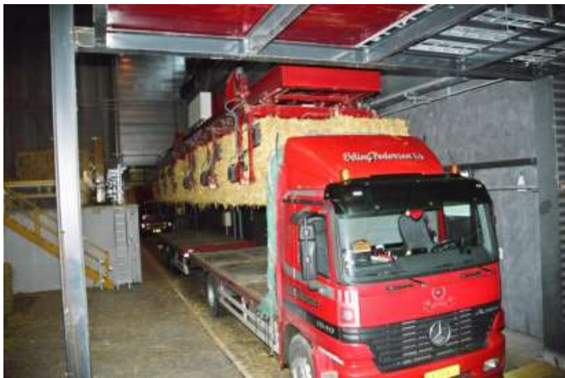
Figure 03-02 14: Unloading straw bales at the Køge Biopellet Factory (Source: mixBioPellets Project)
