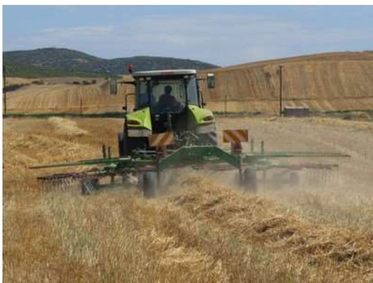
Figure 03-02 2: Windrowing of straw (Source: CERTH)
