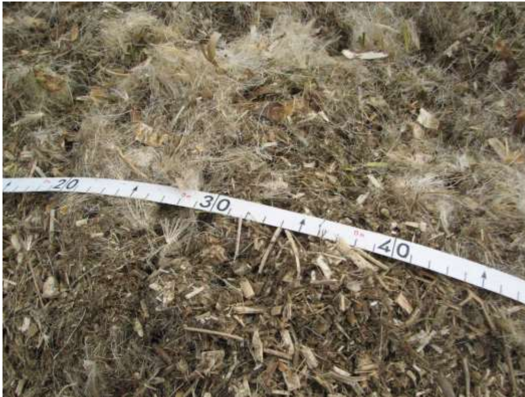
Figure 03-02 9: Cardoon harvested with forage harvester. The inhomogeneous nature of the material is apparent and pieces of stalk, leaves, bracts and seeds can be distinguished. (Source: CERTH)
