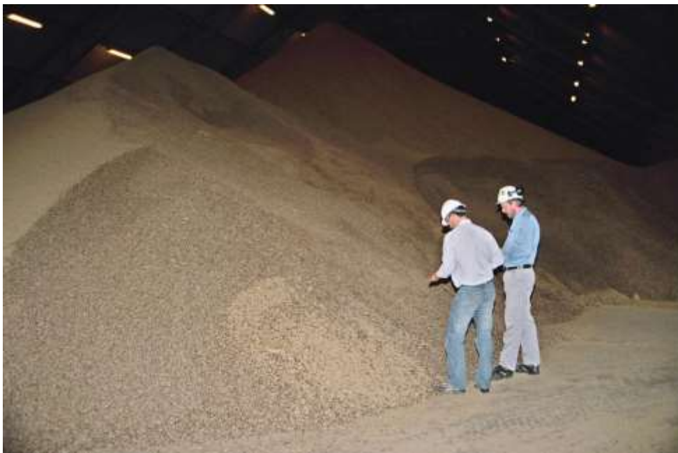
Figure 03-02 8: Bulk storage for straw pellets (Source: mixBioPellets Project)
