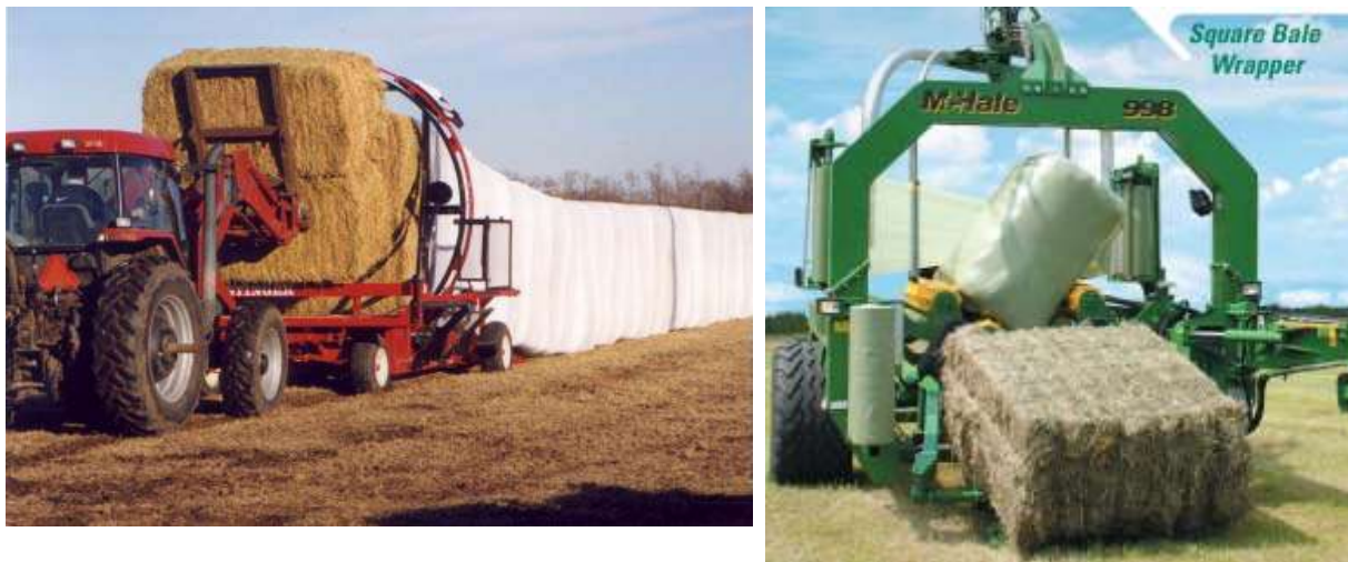
Figure 03-02 6: A tube-wrapped system and stacker, left (Source: University of California) and a square bale wrapper (Source: McHale Engineering Limited)
