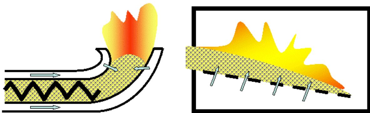
Since the burner is fed from below, using a screw, and the screw feed must be designed so as to prevent back-firing (i.e. that the flames creep backwards through the screw) the feed will be dimensioned as narrow as possible. Hence, the fuel feed will not allow larger or more porous particles to pass and a pellet burner becomes fuel inflexible.
