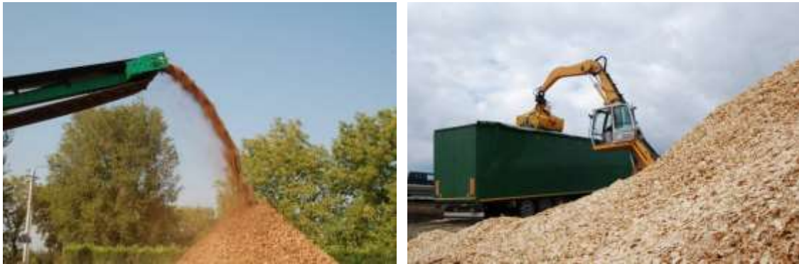
Figure 01-01 5: Behaving as a quasi-fluid wood chips can adapt to different shapes, optimizing transport and storage (source: Picchi)
