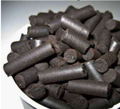
Figure 01-01 12: Pellets from torrefied wood (source: http://www.goforwood.info )
