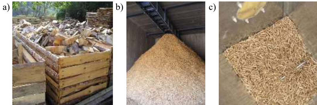
Figure 01-01 14: Size and shape of the single wood particle plays a major role in the definition of bulk density. Loose chunks of wood (a) and wood chips (b) will have a similar bulk volume, while pellets (c) due to their small and homogenous size will have a higher bulk density. (source: Casini)
