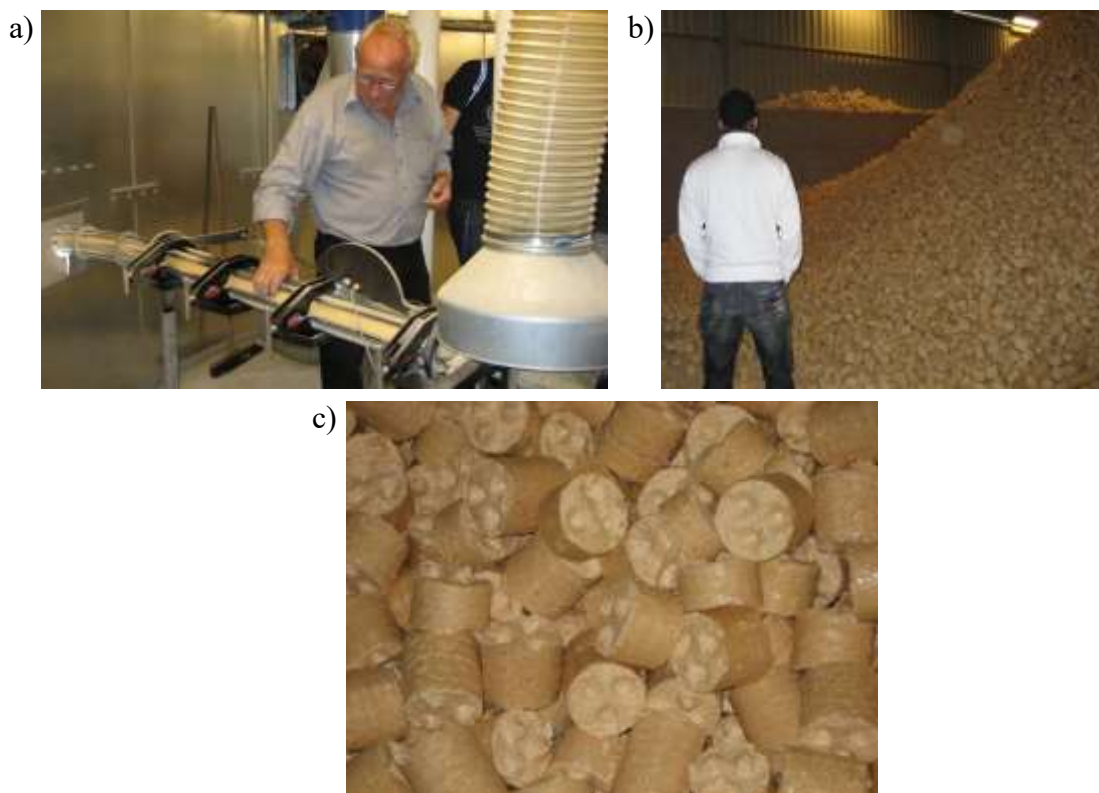
Figure 01-01 11: Briquettes produced from wood dusts; production plant (a), stock of briquettes (b) close-up view of wooden briquettes (c) (source: Zethræus)
