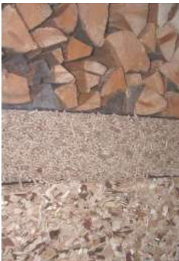
Figure 01-01 13 Direct visual comparison of the three main fuels from woody biomass: woodfuel (above), pellets (centre) and wood chips (below). (source: Picchi)
