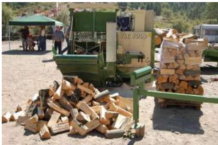
Figure 01-01 2: Wood fuel industrial splitter, note the loose/splitted material and the packaging ready for delivery (right). (source: Picchi)
