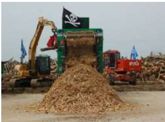
Figure 01-01 9: Wood crusher at work (source: Picchi)
