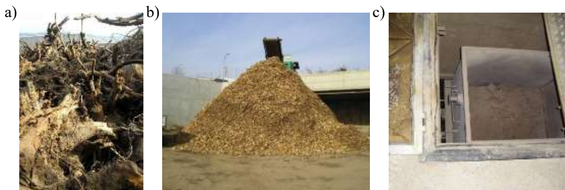
Figure 01-01 17: The stumps of apple trees (a) have a high content of impurities (b) producing large amounts of ashes in the combustion phase (c)
