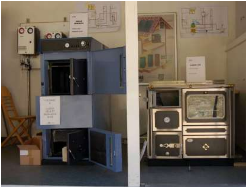
Figure 01-01 3: Two types of wood fuel appliances, a reverse flame boiler (left) and a traditional wood kitchen (right). Note that the size of the loading chamber will influence the size of the wood fuel logs to be used. (source: Picchi)
