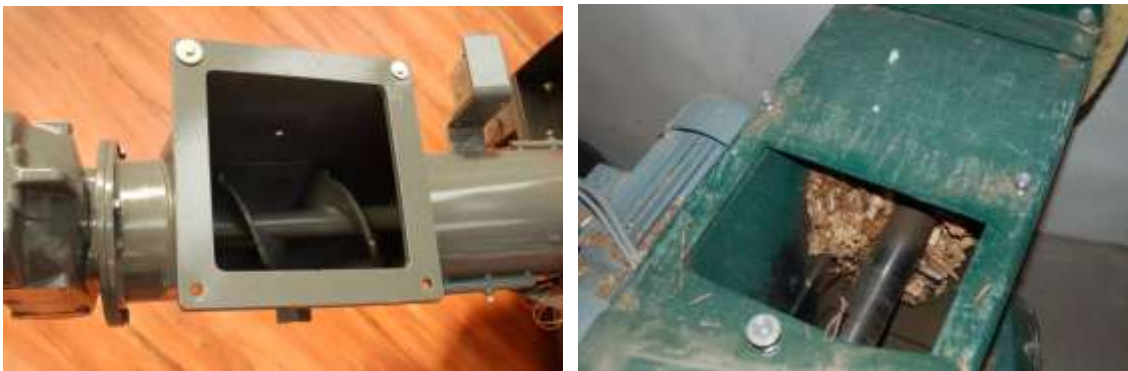
Figure 01-01 6: Examples of screw conveyers for wood chips boilers. This feeding system is very sensitive to chips size, and an irregular fuel with oversized material could jam the screw (source: Picchi)
