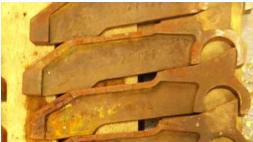
Figure 04-00 8: The grate bars from the side, total length about 30 cm.
