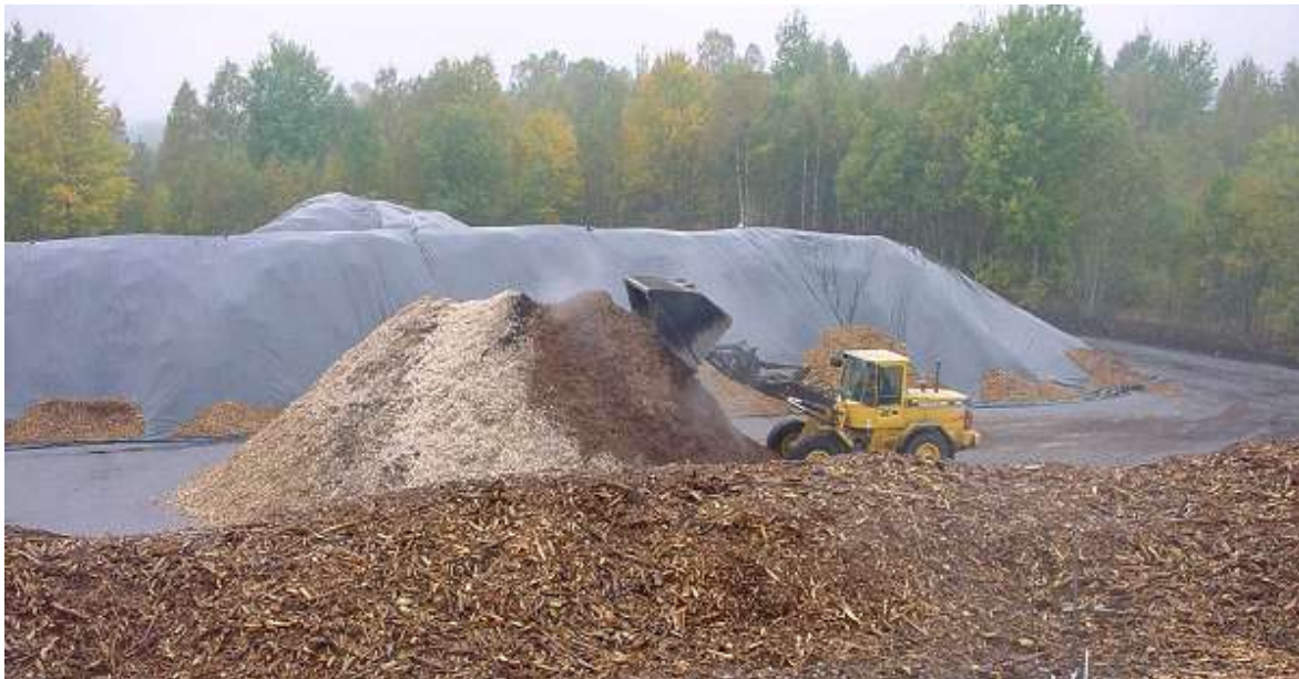
Figure 04-01 3b: Outdoor storage of chips from felling residues at an energy plant
