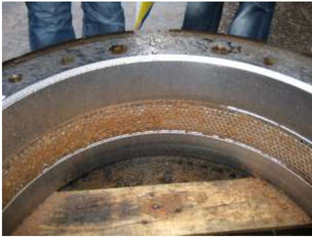
Figure 04-01 5: A worn-out pellet press matrix on a rainy day
