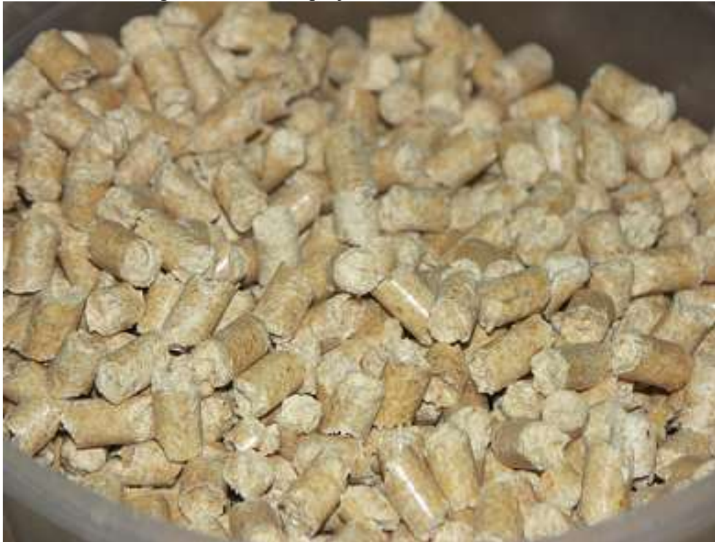
Figure 04-01 4: Wood pellets, about natural size
