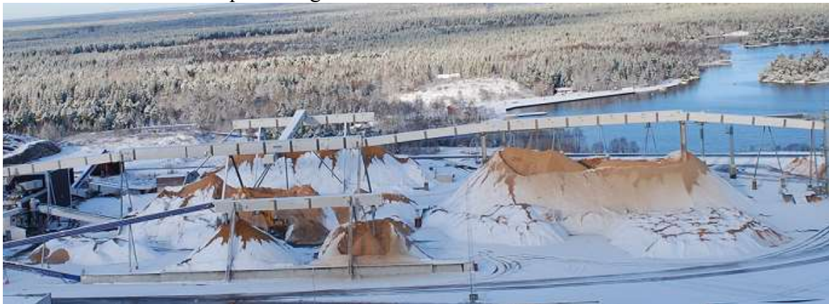
Figure 04-01 3a: Outdoor storage of saw-dust for fuel at a pulp-mill
